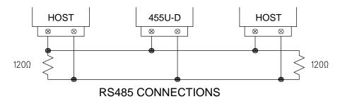
terminated at each end of the network with a 120 ohm resistor. On-board 120 ohm resistors are provided and may be engaged by operating the single DIP switch in the end plate next to the RS485 terminals. The DIP switch should be in the "1" or "on" position to connect the resistor. If the module is not at one end of the RS485 cable, the switch should be off.
