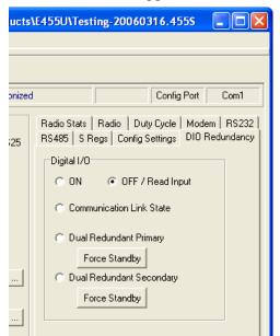
If using Hayes commands, Dual Redundancy is set via the AT#O command ("set output function").
