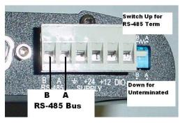
differential standard but it is recommended that shielded, twisted pair cable be used to interconnect modules to reduce potential RFI. It is important to maintain the polarity of the two RS485 wires. An RS485 network should be wired as indicated in the diagram below and
