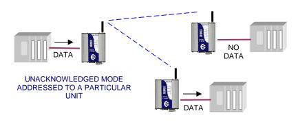
To improve reliability in this mode, units may be configured to send each message multiple times (configured in S-Register S29). The receiving unit will detect repeat messages and only send the data out the serial port once.
