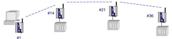
The host protocol is packet based, with message packets of up to 100 bytes. The master station initiates all communication, and waits for a response from the slave devices.
