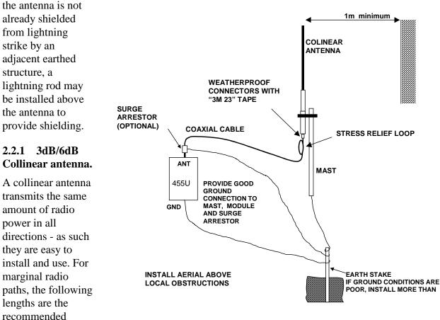
maximum for the coaxial cable to the antenna. RG58 -10 metres RG213 - 20 metres. Note that this applies to marginal paths only - if the radio path has a strong radio signal, then longer
