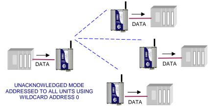
Prior to transmitting, units will listen to the radio channel to ensure that it is clear - units will hold off from transmitting until the radio channel is clear.
