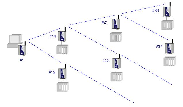
This network has a maximum of three "hops" - to reach the most remote units, there needs to be three transmissions or hops. Unit 1 needs to transmit with address <0,0,0> - that is, three hops.
