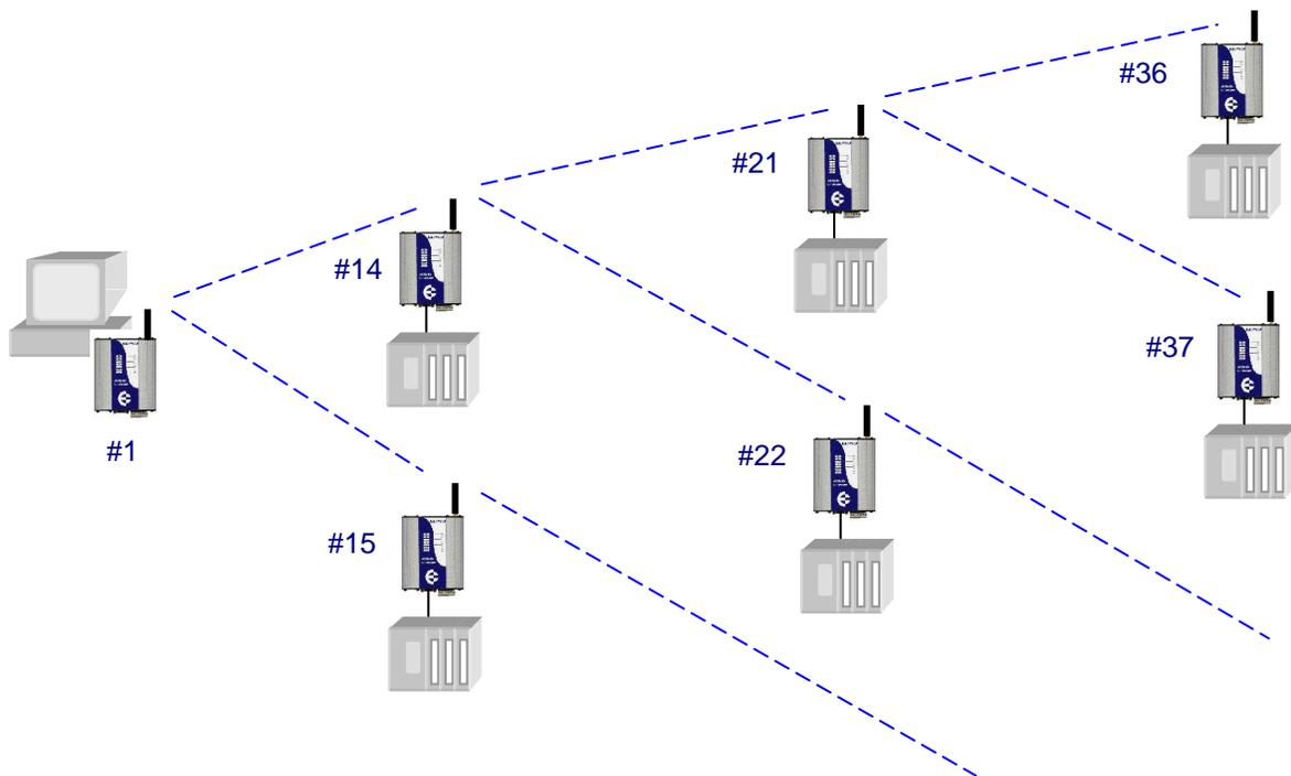
This network has a maximum of three “hops” - to reach the most remote units, there needs to be three transmissions or hops. Unit 1 needs to transmit with address  $\langle 0,0,0 \rangle$  - that is, three hops.
