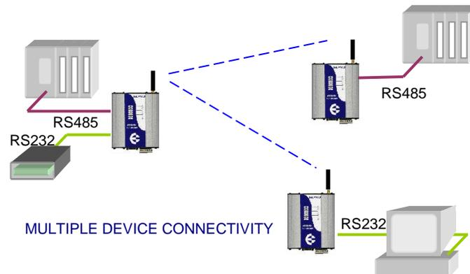
The unit includes a fixed frequency radio transceiver with overall frequency range 360MHz to 512MHz, in seven radio bands, each 20MHz wide. The user can configure the radio frequency within the 20MHz band (refer to Diagnostics section).
