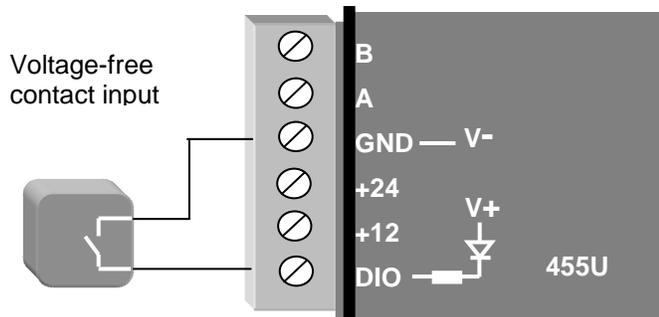
**Note:** The DIO channel is not available when the 455U unit is part of a Dual Redundant pair.
