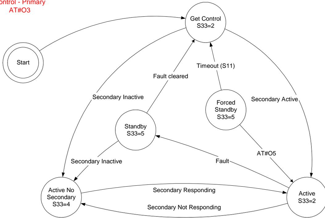
E455U-D Dual Redundant Control - Secondary AT#04
