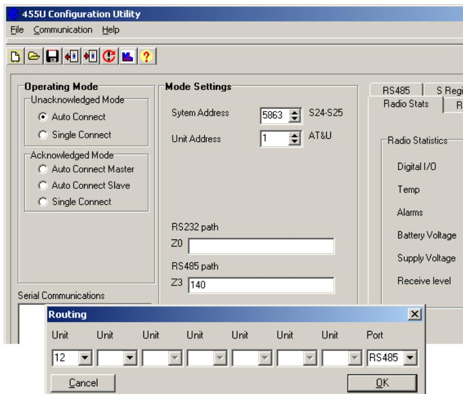
repeater addresses, select the destination module (use the unit address) in the left-hand box. Do not select these boxes. When you click OK, the remote port address is automatically entered into the RS485 path box.
