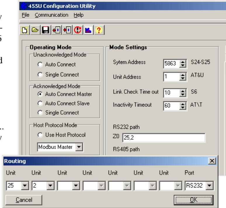
The repeater addresses are entered in order from the master - that is, the leftmost address is the first repeater after the master.
