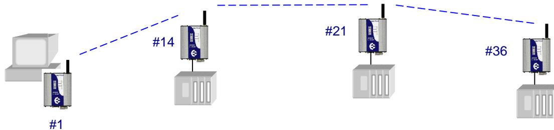
The host protocol is packet based, with message packets of up to 100 bytes. The master station initiates all communication, and waits for a response from the slave devices.
