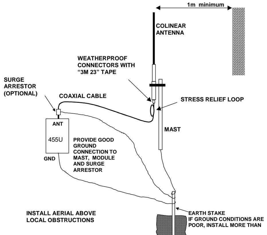
lengths of cable ( and hence more cable loss) can be tolerated. If more than 20 metres of cable is required for a marginal path installation, then a low loss cable such as 10D-FB, or a higher gain antenna should be used. Collinear antennas should be mounted vertically, at least 1 metre away from a wall or mast.
