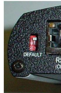
The module will now be configured for 19,200 baud communication on the RS232 DB9 port.
