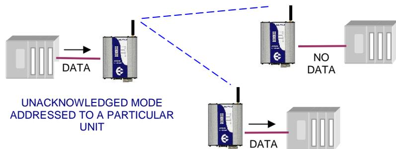
To improve reliability in this mode, units may be configured to send each message multiple times (configured in S-Register S29). The receiving unit will detect repeat messages and only send the data out the serial port once.
