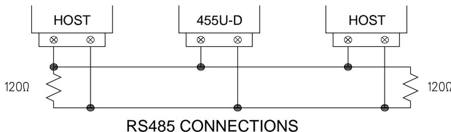
terminated at each end of the network with a 120 ohm resistor. On-board 120 ohm resistors are provided and may be engaged by operating the single DIP switch in the end plate next to the RS485 terminals. The DIP switch should be in the “1” or “on” position to connect the resistor. If the module is not at one end of the RS485 cable, the switch should be off.
