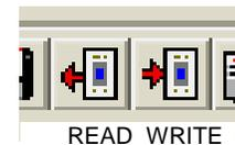
When you read or configure a program, you will see the communication messages between the program and the module in the “Serial Communications” box in the bottom hand corner of the program. The communication messages are Hayes AT commands being generated or read by the program.
