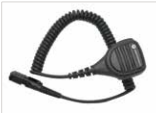
PMMN4075 Small remote speaker microphone, windporting, IP57. No emergency button.
